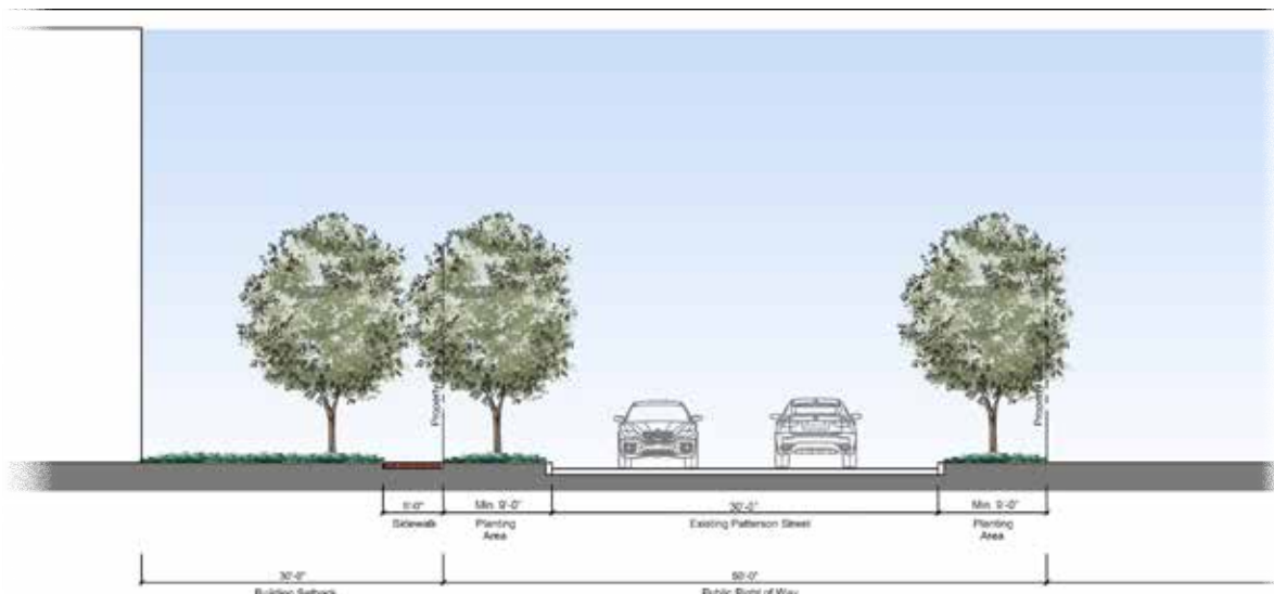
Figure 1: Typical Patterson Street Cross Section
